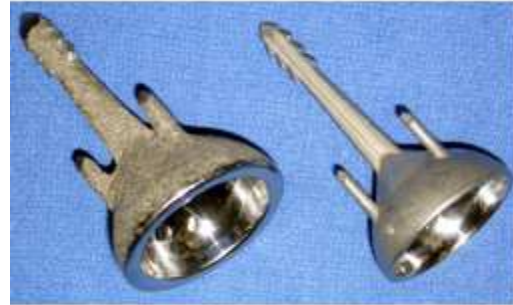
Figure 5 Tronzo Acetabular Components-The prosthesis on the right was used both with and without cement fixation. The component on the left was modified to include a rough surface and was designed for bone ingrowth
