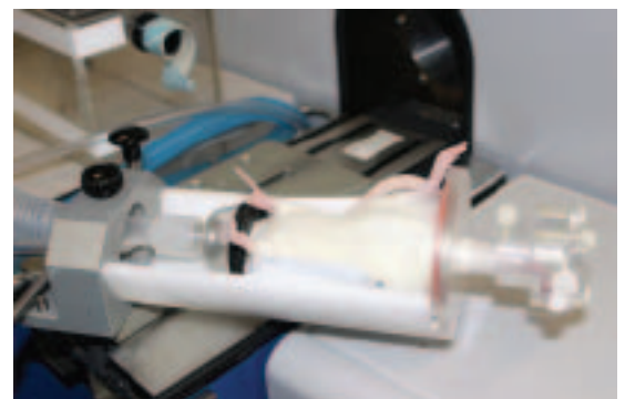
Figure 1. In vivo \mu CT scan of a rat under anesthesia with the right tibia held by customized jig.
