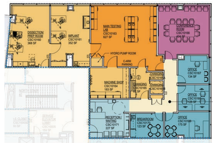
Figure 2. The Biedermann Lab for Orthopaedic Research will have rooms dedicated to dissection and implant placement, along with a main lab testing space to perform biomechanical research. The lab will be located on the 10 th floor of Penn Medicine University City, and will be equipped with five dissection tables, large-scale and small-scale universal testing machines, a mobile C-arm, a 3-D motion capture system, a 3-D printer, and an on-site machine shop.
