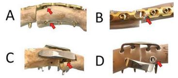
Figure 3. Differences in failure modes for cadaveric and synthetic specimens for the PLT and 2S groups.
