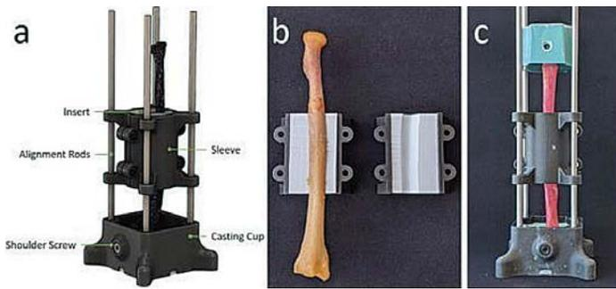
**Figure 2.** (a) 3D model of the radius alignment fixture indicating critical fixture components. (b) Patient-specific 3D-printed insert positions radius in the same orientation as in the virtual model. (c) Radius alignment fixture with an aligned cadaver radius fully potted.
