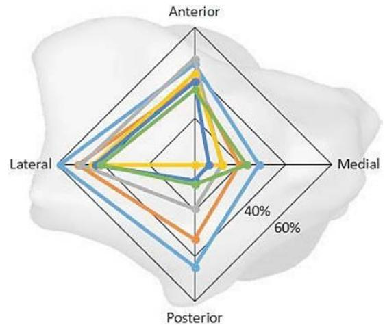
**Figure 3.** Distal-to-proximal view of an aligned radius. Radar chart illustrates the average percent error relative to the aligned condition for all six radii virtually tested under malaligned conditions. Axial stiffness was highly sensitive to malalignment, whereas torsional rigidity was not.
